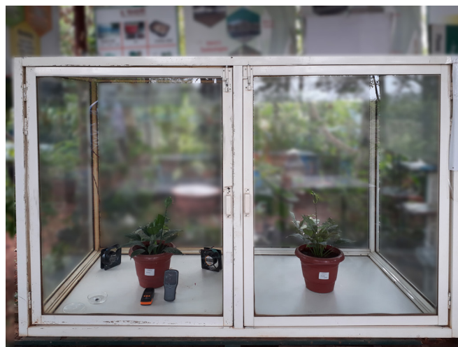
Fig. 2: Treatment chamber with fans and formaldehyde detector
