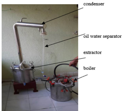
Fig. 1: Experimental Setup for Extraction of Oil
