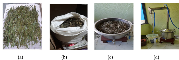
Fig. 7: Experimental Run with 5 kg Raw Material (a) drying, (b) weighing of 5kg, (c) filled raw material, (d) running experiment
