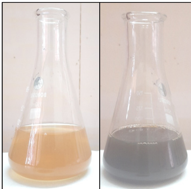
A) Before incubation b) After incubation for 24h Fig. 3: Nanoparticle synthesized of silver plant leaf extract (A, B)
