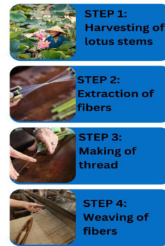
Fig. 1: Process of extraction of lotus stem
