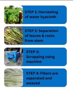
Fig. 3: Process of extraction of fiber from water hyacinth
