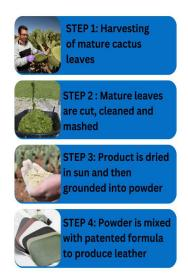
Fig. 2: Process of extraction of leather from Nopal cactus
