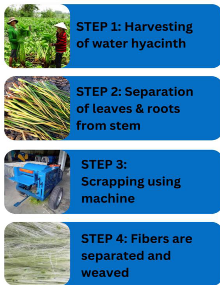
Fig. 3: Process of extraction of fiber from water hyacinth
